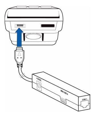
Figure 6 Multiport Adapter Connection to a V<sup>x</sup>670 Terminal
